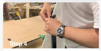
Make sure the metal legs are flat on a table surface and the actylic panel is seated all the way down in the slot.
