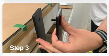
Insert a bolt into the upper hole of the leg and spread a bit as shown on the picture.
