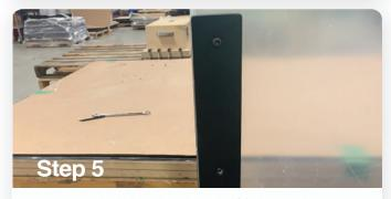
Fit a nut on the bolt on the other side of the leg but do not tighten it yet.
