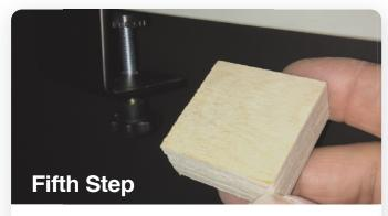
Lightly tighten the clamp Knob under the table. Do not over tighten. Use supplied shims if required.
